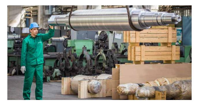
Rolls are usually preserved, packed and shipped in wooden cases or on wooden pallets
